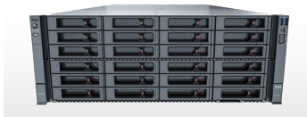
Front backplane of the 5288 V7 (24 drives)
